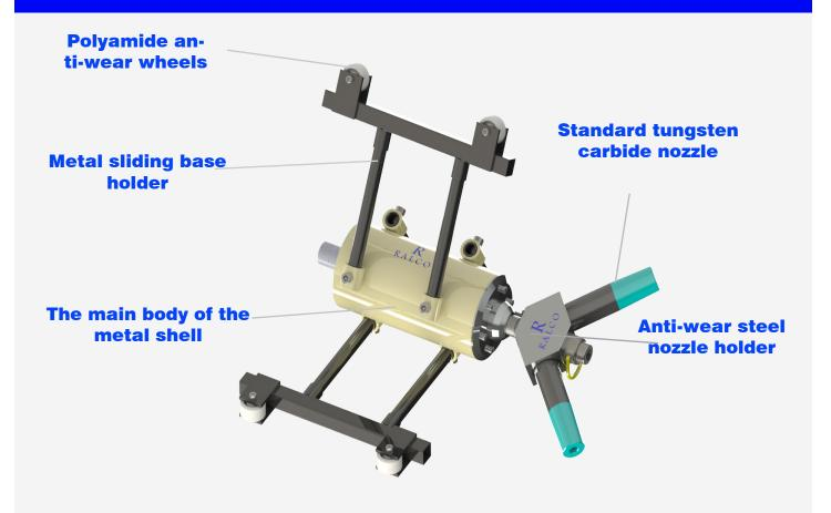
This device is designed for pipes from size 36 inches and above.
